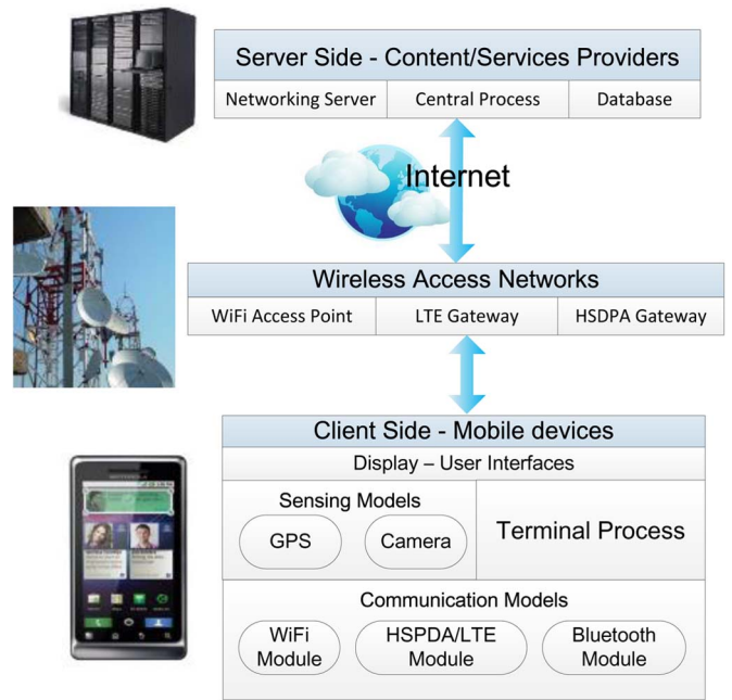
Fig. 2. The physical architecture of the conventional MSNs.
